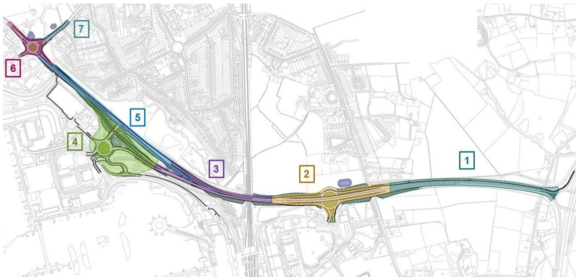
Figure 2.1 : Components of the proposed highway improvements
